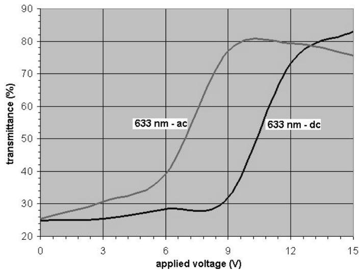
Figure 5. Transmitted intensity versus applied voltage at 633 nm for AC and DC voltages.
