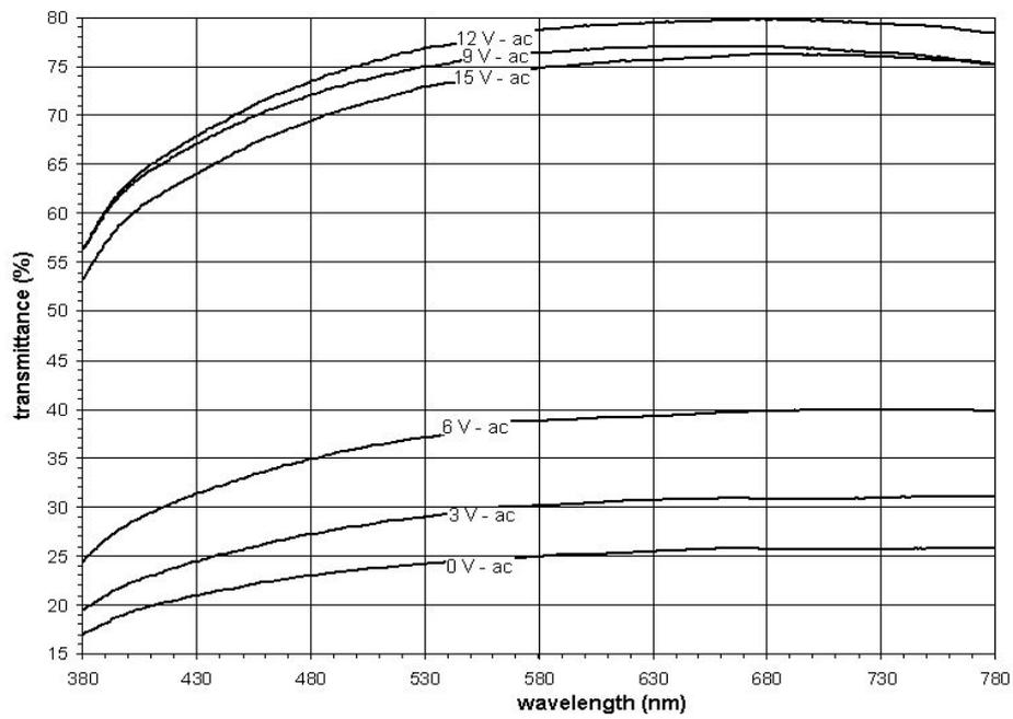
Figure 3. Transmitted intensity versus wavelength under different AC voltages.
